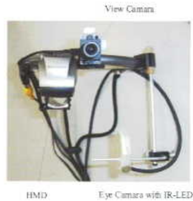
Figure 2. HMD for Eye-gaze Communication (HMD-EC)
